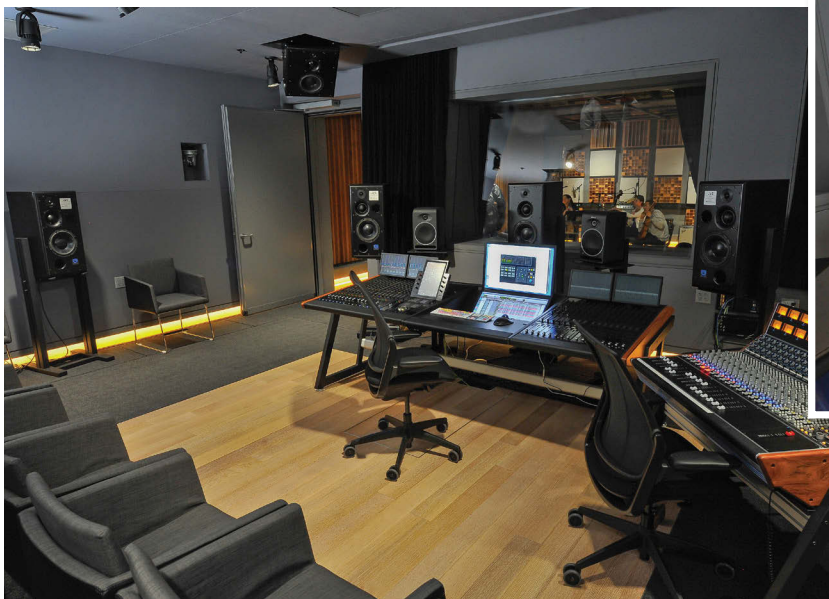
The Marketing Group's Studio C, with Avid S6 and API 1608 consoles, 7.1 ATC SCM50 PSL monitor system and 12 on-wall Triad subs, three per wall. Also, Panasonic PTZ cameras and a Tricaster video switcher for recording or streaming. Inset: John Loose with Erik Foreman and Kevin Perry.
